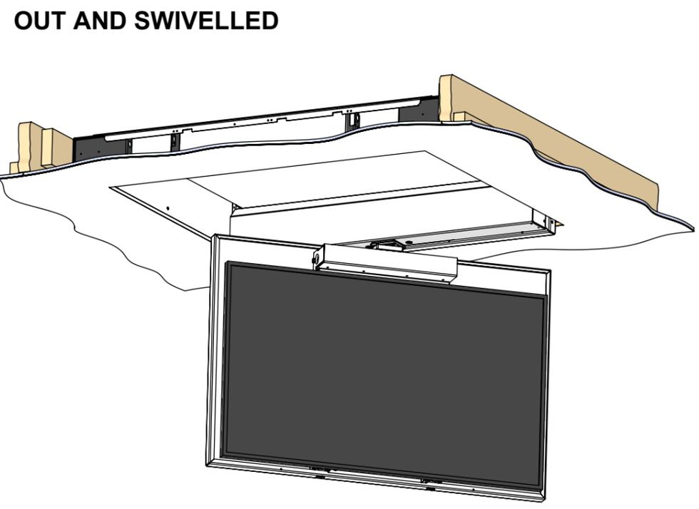
A motorised mechanism to reveal a display from the ceiling. This version hinges down by 90 degrees and then swivels up to 180 degrees of in both directions.
